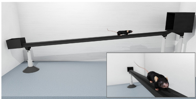
Fig. 1. Rendered image of the tapered beam. The apparatus includes a loading area at the left end and a refuge box at the right end of the beam. Inset: close-up view of a mouse stepping onto the side ledge (foot fault).
